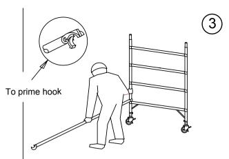
Begin erecting by clipping two horizontal braces as shown ( hooks facing outwards ) to the vertical of the frame.
