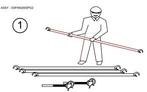
Before erecting the tower ensure site conditions are safe, especially regarding ground and wind conditions. Operatives must be competent and familiarize themselves with this assembly manual. Also make sure sufficient equipment is available to erect required height tower and that components are not damaged or incompatible. Check the component breakdown overleaf for quantities of components required.
