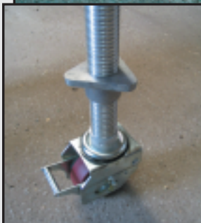
Nut type leg adjustment.
