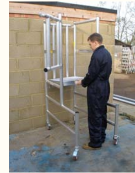
2) PULL GATE OUT BEFORE FITTING PLATFORM
