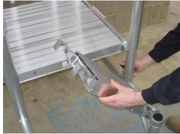
3 ) RELEASE STEP LOCK BOLT AND LOWER STEP OR LOCATE INDIVIDUAL STEP
