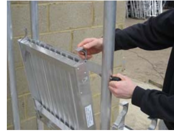
2 ) RELEASE PLATFORM LOCK BOLT AND LOWER PLATFORM OR LOCATE INDIVIDUAL PLATFORM
