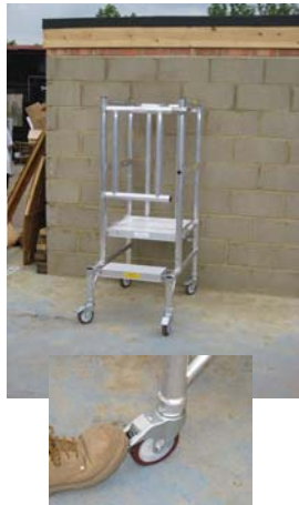
5 ) LOCATE PODIUM AND LOCK CASTORS
