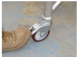
LOCATE UNIT AND LOCK ALL CASTORS
